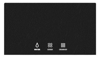
**Sleep Mode** displays only the WATER, CUBES and CRUSHED options. Touch an icon to activate the desired dispenser mode. The active dispenser mode is more brightly illuminated.
