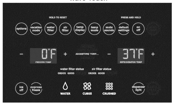
Your refrigerator is equipped with a Wave-Touch™ control panel display. It is only necessary to gently touch the glass. There are three (3) levels of display.
