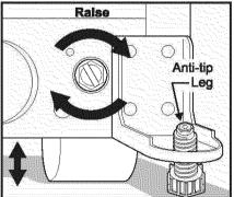
5 After unit is leveled, lower anti-tip leg until it contacts the floor.
