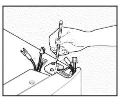
2 Disconnect the harness by grasping both sides of the connector firmly, depress the latch, and pull apart. Remove the two (2) screws from the top hinge. Lift the door off of the bottom hinge and set it aside.
