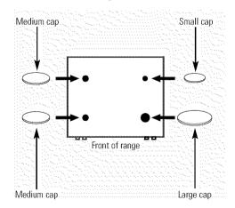
Make sure that the heads and caps are replaced in the correct locations.
