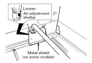
On some models, remove the metal shield at the rear of the cavity.
