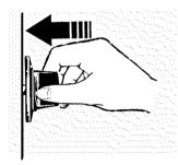
Push the control knob in and turn it to the **LITE** position (on electric ignition models) or **HI** (on standing pilot models).
