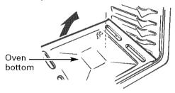
**4.** Locate the pilot in the back of the oven bottom. The pilot is attached to the left side of the oven burner.
