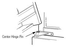
Lift the top hinge so the pin fits into the door
