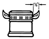
Typical surface burner flame at highest setting
