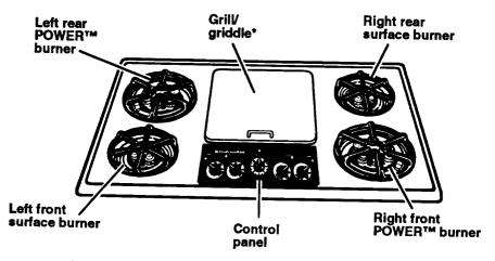
\*Includes brushed chrome cover with handle, stick-resistant commercially finished grill, stick-resistant commercially finished griddle, porcelain flavor generator insert, and porcelain drip pan.
