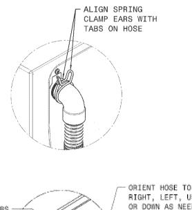
TABS RIGHT, LEFT, UP OR DOWN AS NEEDED BEFORE PLACING CLAMP IN POSITION ALWAYS ALIGN CLAMP EARS WITH TABS ON HOSE
