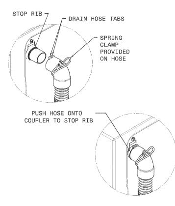
3. Using pliers, squeeze the ears of the spring clamp and position the clamp so the clamp ears <u>align with</u> <u>and contact the tabs</u> on the drain hose. This assures proper location of the clamp to prevent leaks.
