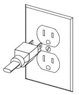
accessible when the washer is in an installed position. *NOTE:* GFI (Ground Fault Interrupter) receptacle is not required.
