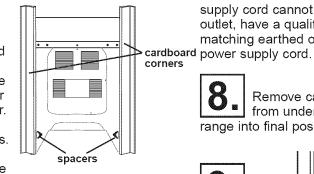
floor in back of range so corners will support outer side edges of range as shown.
