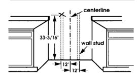
To mount anti-tip bracket to wood or metal wall stud: Find the wall stud that is closest to the center of the range location. (Note: Wall stud should Not be more than 12 inches to the right or left of center of range location.) Measure and mark at the center of the wall stud a distance of 33-3/16 inches up from the floor.
