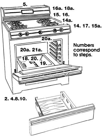
■ Use pipe-joint compound made for use with Natural and L.P. gas to seal all gas connections. If flexible connector is used, be certain connector is not kinked.
