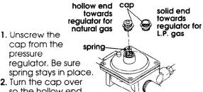
2. Turn the cap over so the hollow end faces outward.
