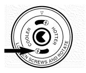
The lower screw moves toward COOLER to decrease the temperature.
