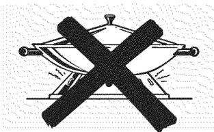
Do not use a flat-bottomed wok on a support ring. Placing the ring over the burner or grate may cause the burner to work improperly, resulting in carbon monoxide levels above allowable standards. This could be dangerous to your health.
