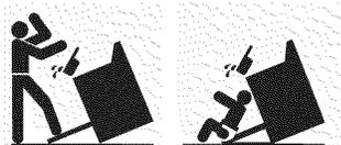
**▲ WARNING:** If your range is removed for cleaning, servicing or any reason, be sure the anti-tip device is reengaged properly when the range is replaced. Failure to take this precaution could result in tipping of the range and cause injury.
