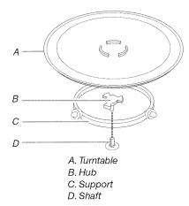
The turntable can rotate in either direction to help cook food more evenly. For best cooking results, do not operate the microwave oven without having the turntable in place. See "Assistance or Service" to reorder any of the parts.
