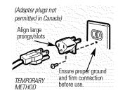
The larger slot in the adapter must be aligned with the larger slot in the wall receptacle to provide proper polarity in the connection of the power cord.
