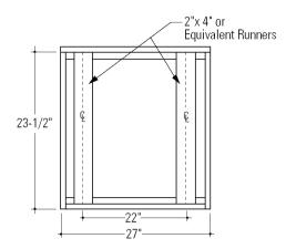
**IMPORTANT:** When installed below a single or double oven, check to be sure that any oven supports above the cutout do not obstruct the 23-1/2" required depth of the warming drawer cutout.
