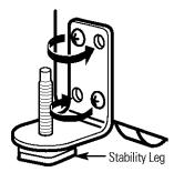
Install the bottom hinge bracket on the left side.
