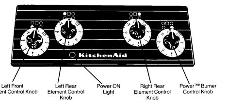
The white circle in the diagram above each knob indicates which element that particular knob controls.
