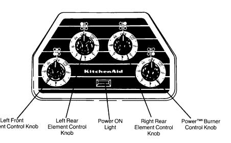
The white circle in the diagram above each knob indicates which element that particular knob controls.
