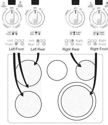
Fig. 2 (Bridge Element on some models)
