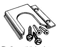
The floor anti-tip bracket MUST be installed. To install the anti-tip bracket shipped with the range, see Panels D and E and the anti-tip bracket template.
