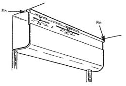
**3.** Pull the bottom of the light shield down and forward, then rotate the top up and off.
