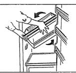
7. If tape holds bottom drawer cover to drawer supports, remove the tape. Pull drawer partway out. Reach in, push the rear of the glass up and, at the same time, back, until it clears front-corner retainers.
