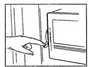
Set the control lever all the way down to convert the drawer to normal refrigerator temperature and provide extra vegetable storage space. The cold air duct is turned off.
