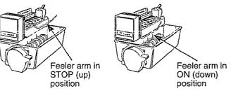
When the water supply has been connected to the icemaker, move the feeler arm to ON (down) position.
