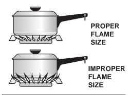
Never extend the flame beyond the outer edge of the utensil. A higher flame simply wastes heat and energy, and increases your risk of being burned by the flame. **For most cooking**, start on the highest control setting and then turn to a lower one to complete the process. Use the recommendations below as a guide for determining proper flame size for various types of cooking. The size and type of utensil used and the amount of food being cooked will influence the setting needed for cooking.
