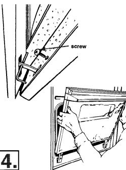
Close lower oven door to the broil position. Grasp the sides of the oven door and pull the door up and out of the hinge slots to remove . Set door aside.
