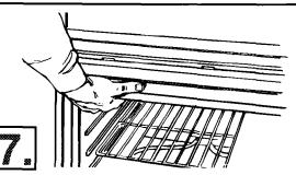
Remove and discard shipping base. Lift oven up into cabinet cutout using the oven opening as an area to grip.
