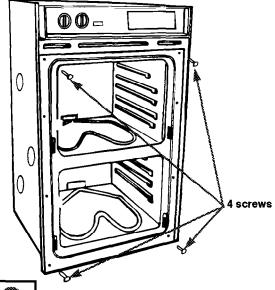
8. Center oven into cabinet cutout. Use two screws (four screws for a double oven) through the mounting holes in the front frame of the oven to secure the oven to the cabinet. Do Not overtighten screws.
