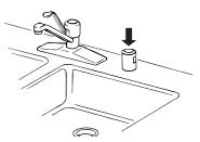
The drain air gap is usually located on top of the sink or countertop near the dishwasher. To order a drain air gap contact your local dealer, or in the U.S.A., call the Consumer Assistance Center at 1-800-253-1301 and ask for Part Number 300096.
