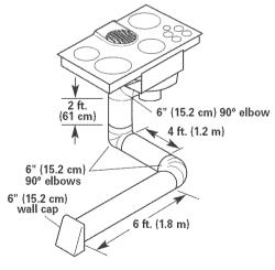
90° elbows (3) = 15 ft. (4.6 m) 12 feet (3.7 m) straight = 12 ft. (3.7 m) Wall cap = 0 ft. (0 m) Equivalent length of = 27ft. (8.3 m)
