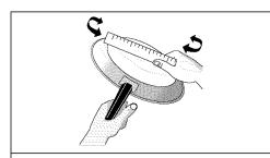
Pans should have flat bottoms that make good contact with the entire surface element. Check for flatness by rotating a ruler across the bottom. There should be no gap between the pan and ruler.
