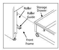
To open the storage drawer, push the drawer in gently and it will spring open. To close, push the drawer until you hear a click, which indicates that the spring is compressed, and the drawer is closed.
