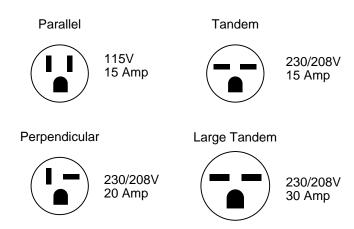
**Wall Outlets:** All wiring including installation of receptacle must be made in accordance with local electrical codes and regulations. Electrical outlet should be in reach of line cord.
