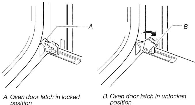
3. Grasp the edges of the oven door with both hands and close the oven door until it will no longer close. Lift and pull oven door toward you and remove. Set the oven door(s) aside on a covered work surface.
