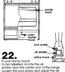
Loosen the lock screw and adjust the air shutter until the proper flame appears. Tighten screw.
