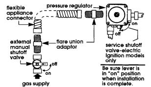
Pull range forward to make gas connections. Assemble the flexible connector from the gas supply pipe to the pressure regulator, located on the lower right hand side on the back of the range, in this order: shutoff valve, 1/2" flare union adapter, flexible connector, 1/2" flare union adapter. Seal all openings in floor or wall wherever range is installed.
