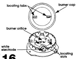
**6** ■ Align locating tabs on burner caps with locating slots in burner base. Burner cap should be level when properly positioned. Place burner grates over burners and caps.
