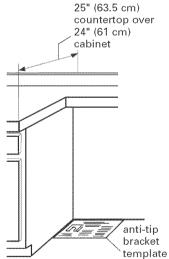
Place the anti-tip bracket template on the floor in the cabinet opening so that the left edge is against cabinets and the top edge is against the rear wall, molding or cabinet.
