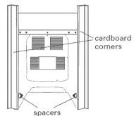
Take 4 cardboard corners from the carton. Stack one cardboard corner on top of another. Repeat with the other two corners. Place corners lengthwise on the floor in back of range so corners will support outer side edges of range as shown.
