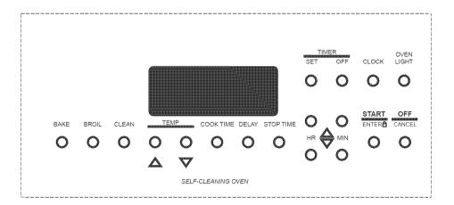
Check the operation of the oven burner. Push the "BAKE" pad and "Pre'F" will appear in the temperature display. Press the "Start/Enter" pad. A preheat time will count down. The oven burner should light in 50 to 60 seconds. This delay is normal. The oven safety valve requires a certain time before it will open and allow gas to flow.
