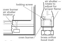
26 If the oven flame needs to be adjusted, locate the air shutter near the center rear of range. Loosen the locking screw and rotate the air shutter until the proper flame appears. Tighten locking screw.
