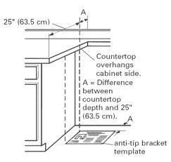
If countertop opening is deeper than 25 inches (63.5 cm), measure and mark a distance 25 inches (63.5 cm) in from front of countertop opening and align template with mark (or subtract 25 inches (63.5 cm) from countertop depth and add the difference to the corresponding dimension).
