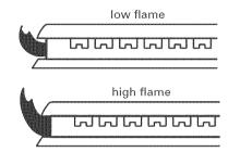
Adjust the height of top burner flames (some models). The cooktop LOW burner flame should be a steady blue flame approximately 1/4" (0.64 cm) high. It can be adjusted using the adjustment screw in the center of the valve stem. The valve stem is located directly underneath the control knob.
