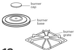
■ Remove cooktop burner caps and grates from parts package. Align notches in burner caps with pins in burner base. Burner caps should be level when properly positioned. Place burner grates over burners and caps.
