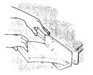
To remove the screen, open the lid door and pull the screen straight out. Roll the lint off the screen with your fingers. **DO NOT rinse the screen or wash it.** Wet lint is hard to remove. When replacing the screen, push it firmly into place. Close the lid. BEFORE USING/CONTENTS/LOADING/LINT SCREEN
