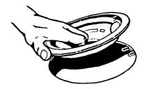
3. Hold the surface unit as level as possible with the terminal just started into the receptacle. Push the surface unit terminal into the receptacle.
