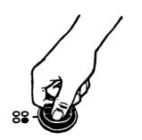
2. Line up openings in the drip bowl with the surface unit receptacle and the element hold-down clip.
