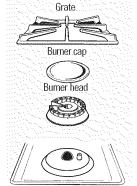
cap. Replace the side grates so that they fit over the tabs on the vent grille. Make sure the grates are positioned securely over the burners and that they are stable and level.
