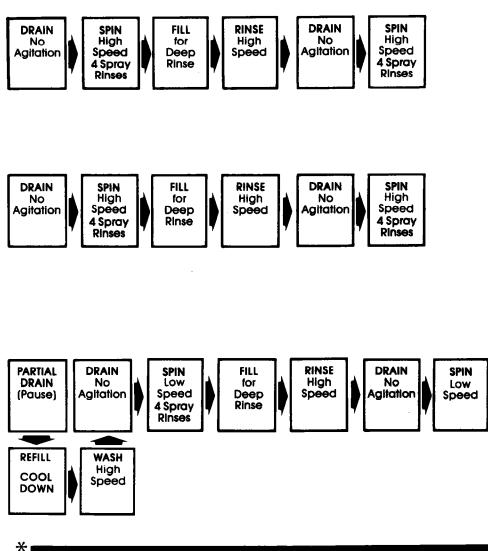
IMPORTANT: THE WASHER WILL PAUSE BRIEFLY THROUGHOUT EACH CYCLE. These pauses are normal. They allow for the reversing of the motor, normal washer operations, and the cool down portion of the PERMANENT PRESS Cycle.
