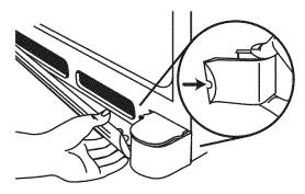
Using a screwdriver or %" hex driver, turn the roller adjustment screw on each side to raise or lower that side of the refrigerator.
