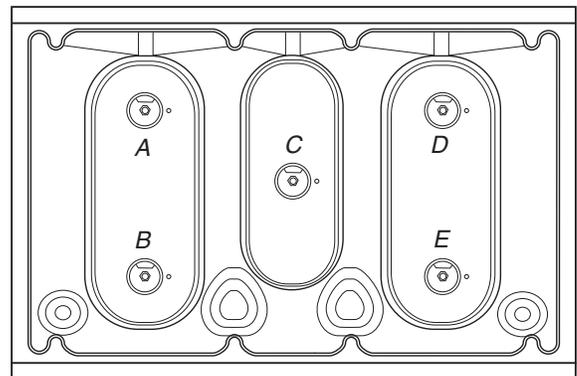
A. Standard burner - LP gas orifice spud number 78
