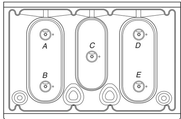
A. Standard burner - Natural gas orifice spud number 125
