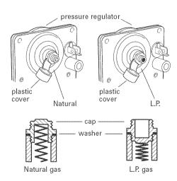
Surface burners: Remove burner caps. Use a Phillips or Quadrex screwdriver to remove the two screws holding the burner head down. Lift the burner head off the cooktop to uncover the orifice spud holder. The orifice spud is recessed in the holder.
