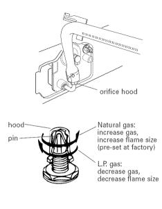
**5** Broil burner: Use 1/2" combination wrench to loosen orifice hood away from pin (approximately 2 to 2-1/2 turns). The burner flame cannot be properly adjusted if this conversion is not made.
