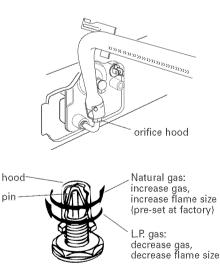
**5** Broil burner: Use 1/2" combination wrench to turn the orifice hood down snug onto pin (approximately 2 to 2-1/2 turns). Do not overtighten. The burner flame cannot be properly adjusted if this conversion is not made.
