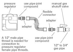
**10** Use 5/16" combination wrench and channel lock pliers to attach the flexible connector to the adapters. Check that connector is not kinked.
