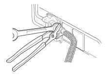
**1** Check that range regulator shutoff valve is in the "on" position. Open the manual shutoff valve in the gas supply line.
