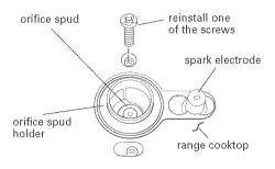
Locate the Natural gas orifice spuds on the spud card on the back of the range. Orifice spuds are stamped with a number and marked with two color dots.
