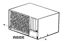
Attach the front grille to the case by inserting the tabs on the grille into the slots on the front top of the case. Push the grille in until it snaps into place around the power cord on the right side.
