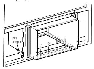
H Pull the accordion panels to each window sash track. Attach them on each side to the window sash and the window stool using 4 type B screws.
