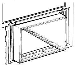
**NOTE**: Do not shut the window so tightly that movement of the accordion panels is restricted.
