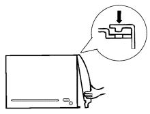
Secure the front grille to the case by replacing the 3 screws removed earlier.
