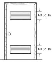
When louvers or registers are placed in door openings, the free air openings of the louvers or registers must equal 120 square inches.
