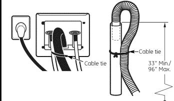
**NOTE:** Drain hose MUST be secured to drain facility in all cases.
