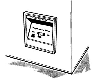
The Temperature Alarm (located on the lower right front of the freezer) works together with an electronic Temperature Sensor (located inside the freezer – sensing freezer temperature) to alert the user to an abnormal condition which has caused freezer temperature to rise to a level which may be unsafe for frozen food storage. It is designed to sound a continuous tone if the freezer becomes warm.
