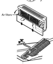
5. Reinstall the air filter dried at the shade and then close the panel.
