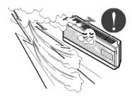
Do not open the inlet grill of the product during operation. (Do not touch the electrostatic filter, if the unit is so equipped.)
