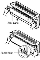
3. Come down the panel and then remove the air filter.
