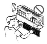
Do not block the inlet or outlet of air flow.
