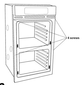
**6** ■ Important: Securely fasten oven to cabinet using the screws provided (two screws for a single oven or four screws for a double oven). Insert the screws through holes in mounting rails. Do Not overtighten screws.
