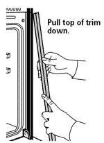
■ Remove trim screws attaching right and left side trim to oven. Grasp the bottom end of trim and pull away from oven. Slide top end of trim downward to remove trim from oven. Take care not to scratch other surfaces with ends of trim. Set trim and screws aside on protected surface.
