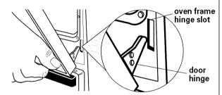
Replace the single or upper oven door by inserting ends of hinges into hinge slots in oven frame. Push behind each hinge so that hinges are pushed into oven frame as far as they will go. Open door and remove both door removal pins. Close and open door to check that door closes and opens completely. If door does not close or open completely, you have not pushed hinges completely into frame. Repeat door removal step and reinsert door into hinge slots again.
