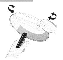
Cookware should have flat bottoms that make good contact with the entire surface heating element. Check for flatness by rotating a ruler across the bottom of cookware. Be sure to follow the recommendations for using cookware has shown in figure aside. \*GOOD
