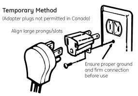
**ACAUTION:** Attaching the adapter ground terminal to the wall receptacle cover screw does not ground the appliance unless the cover screw is metal, and not insulated, and the wall receptacle is grounded through the house wiring. The customer should have the circuit checked by a qualified electrician to make sure the receptacle is properly grounded.
