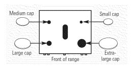
Make sure that the heads and caps are replaced in the correct locations.
