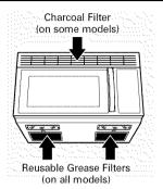
The vent fan has 2 metal reusable grease filters.
