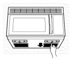
**To remove,** slide it to the rear using the tab. Pull it down and out.
