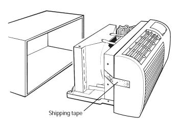
**2** Remove the room cabinet by pulling it out at the bottom to release it, then lift it up to clear the rail along the unit top.
