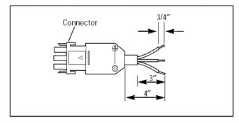
5 Strip 3/4'' of the insulation away at the end of each of the three wires (L1, Neutral and Ground). Plug the connector fully into place in the chassis mating connector. Be sure the locking tabs at the sides are engaged.
