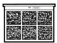
Clogged filter—Greatly reduces cooling, heating and airflow.
