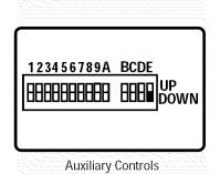
Switch E controls the Freeze Sentinel. When the switch is **DOWN** the Freeze Sentinel automatically turns on the resistance heater and fan if the room temperature (sensed at the unit) drops to approximately 40° F. It will turn the heater off when the temperature reaches about 45° F.
