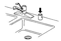
The drain air gap is usually located on top of the sink or countertop near the dishwasher. To order a drain air gap call your local dealer, or in the U.S.A., call the Customer Interaction Center at 1-800-422-1230 and ask for Part Number 300096.
