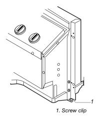
**4.** Loosen the 2 screws on the bottom of each side bracket. **NOTE:** Do not remove these screws.
