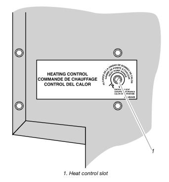
The heating control is located behind the front cover on the right side panel of the chassis. Its function is to allow you to set the outdoor temperature range in which the heat pump operates. This control switches the unit heating supply mode between the heat pump and electric resistance heat based on the outdoor ambient temperature. These changeover temperatures are based on the settings of the control. The factory setting is at the one o'clock position.
