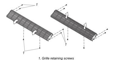
The indoor air discharge grille can be positioned to direct the air either straight up or at an angle into the room.
