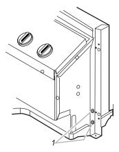
1. Side-bracket screws-loosen; do not remove
