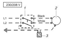
\_\_ \_ Field Supplied Wiring
