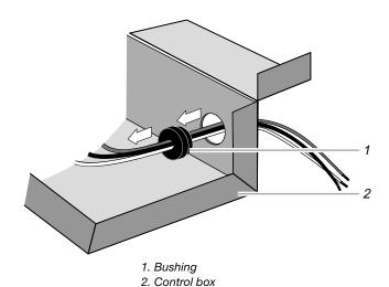
11. Install field-supplied conduit into the same hole as the original bushing for the chassis pigtail wires on the control box.
