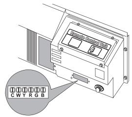
Connect the field supplied 5 or 6 conductor, NEC Class 2, 24 volt thermostat wire to the terminals in accordance with the wiring diagram.
