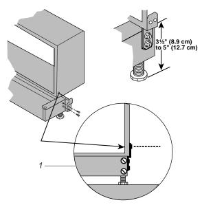
Align, center punch and drill two 5/2 in. holes in wall sleeve.
