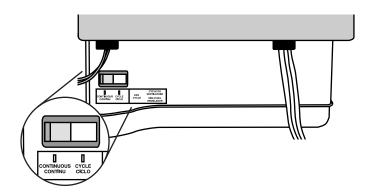
On standard models with unit-mounted controls, the fan cycle switch is located behind the front cover. It is designed to operate the fan either continuously or intermittently. When the switch is in the CONTINUOUS position, the fan will run continuously at the selected speed when the unit is turned on. With the fan cycle switch in the CYCLE position, the fan will run only when the compressor or heating elements cycle on.
