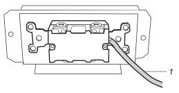
1. Ground wire to subbase ground lug
