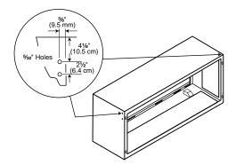
6. Use the seal plates on the chassis as templates. Align the bottom edge of the seal plate against the slanted edge of the deck, and align the side with the outer edge of the cutoff flange. Mark the location of the holes, center punch and drill two ½ in. holes through the flanges on each side.
