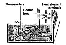
Electric dryer with back panel removed
