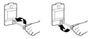
**STEP 3.** Turn bulb couterclockwise. Replace the bulb with a 10-watt appliance bulb only. Replace the cover and secure with the screw.
