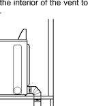
Terminate the exhaust vent outside. The exhaust vent must not terminate beneath the mobile home and must not be connected to any other duct, vent or chimney.
