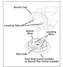
**CAUTION** Use caution when replacing the burner cap so the electrode is not damaged. This may cause a delayed ignition or prevent the burner from igniting.
