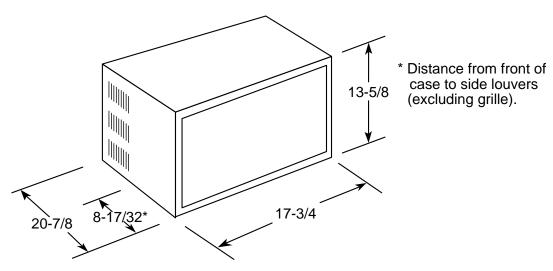
**Note:** When installing units in through-the-wall applications, keep louvers free. Do not restrict air flow areas. Fixed chassis units are not designed for through-the wall applications.
