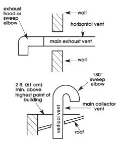
**Do Not** install screening or cap over end of vent.
