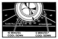
The PERMANENT PRESS Cycle has 10 minutes of cool down time at the end of the cycle.
