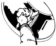
Non-colorfast items can stain the drum. Wipe **carefully** after drying to make sure there is no dye to be transferred to items in the next load.
